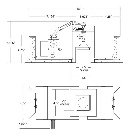
Provided with two (2) 14 gauge steel butterfly type brackets for black iron installations.
